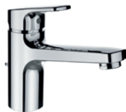
CITYPRO / CITYPRO LIBERTY HF500943100000 Basin mixer, projection 140 mm, fixed spout, Eco+ function, with pop-up waste, chrome
