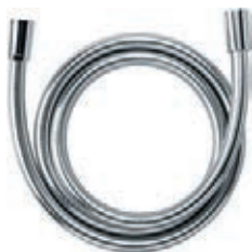
WI504740000000 Simiflex flexible hose 1/2" x 1/2", with me- talic effect and swivelling connection, hose length 1250 mm
